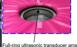
Full-ring ultrasonic transducer array
